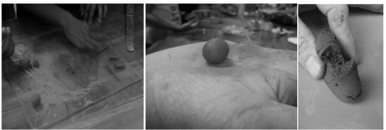
Figure 1.3: Dry Strength Test
