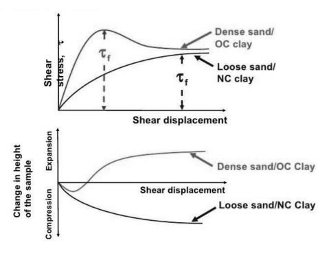
Figure 11.2 Stress-strain relationships of sand (Direct Shear Test)
