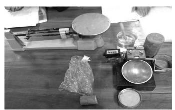
Figure 7.3: Atterberg Limit Test Apparatus
