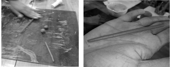
Figure 1.4: Toughness and plasticity Test
