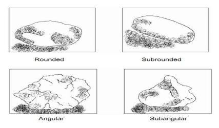
Figure 1.1 Shapes of coarse-grained soil particles
