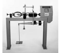
Figure 11.1 Direct Shear Test device of the laboratory
